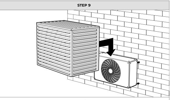
Place the enclosure over the air conditioning/heat pump onto the expansion bolts.
